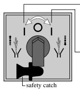
**left position:** cutting rollers run **backwards** and release blocked shredding material
